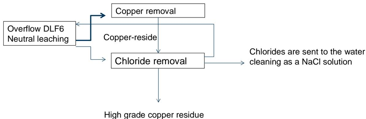
**Figure 2:** Simplified flow sheet for the chloride removal.
